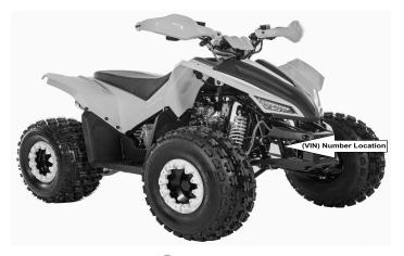
The vehicle identification number (VIN) can be found on the right side of the vehicle behind the front bumper engraved on the frame.
