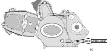
The engine number can be found on the bottom left of the crank case .
