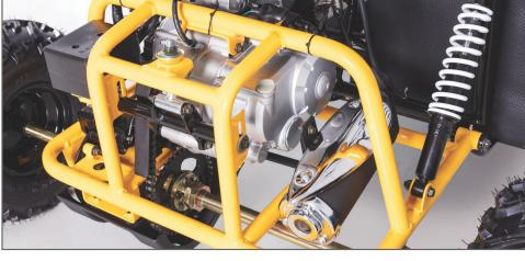
Engine Type Start Type Transmission GY6 169cc Air-cooled Four-strokeCylinder Electric Start Chain Drive Engine Gear Gear Selector Lever Fully Automatic with reverse D-N-R Hand CDI Ignition
